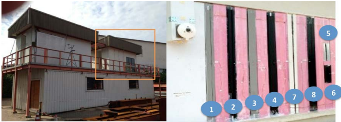
Figure 10. a) Site of the test installation used to obtain the physical temperature measurements of window frame temperature during natural weather exposure in Singapore. b) The outdoor view of the completed frame installation. The window opening was replaced with multiple frame samples so all frame samples were exposed together. Key: 1. Light color non-thermally broken frame, 2. Dark color non-thermally broken frame, 3. Light color, low performance thermally broken frame, 4. Dark color, low performance thermally broken frame, 5. Light color medium performing thermally broken frame, 6. Dark color, medium performing thermally broken frame, 7. Light color, high performance thermally broken frame, 8. Dark color, high performance thermally broken frame (SERIS 2014).
