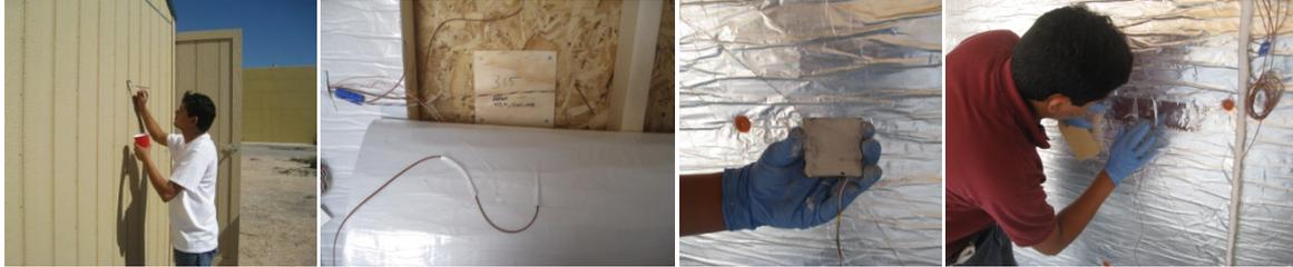
**FIGURE 3: Installing temperature and heat flux sensors. Left to right: temperature sensor on exterior wall, heat flux sensor on interior side of OSB and thermocouple array through assembly, and installing heat flux sensor on reflective insulation with reflective tape.**
