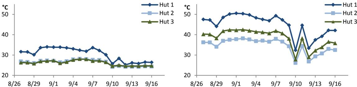
**FIGURE 5: Daily peak air temperatures: LEFT=conditioned zone; RIGHT=unconditioned attic.**
