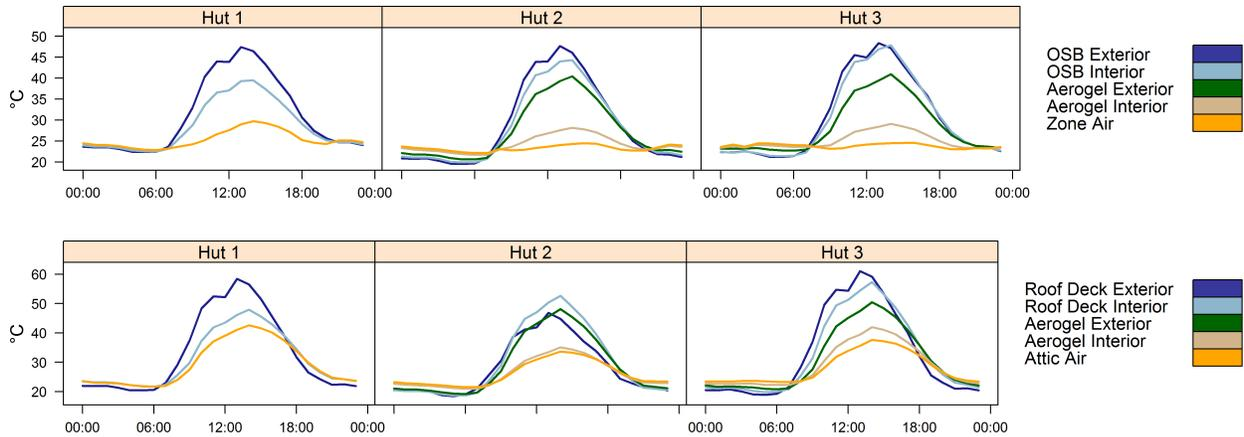
**FIGURE 6: Temperature profile across south wall (top) and roof assembly (bottom) for sample day.**
