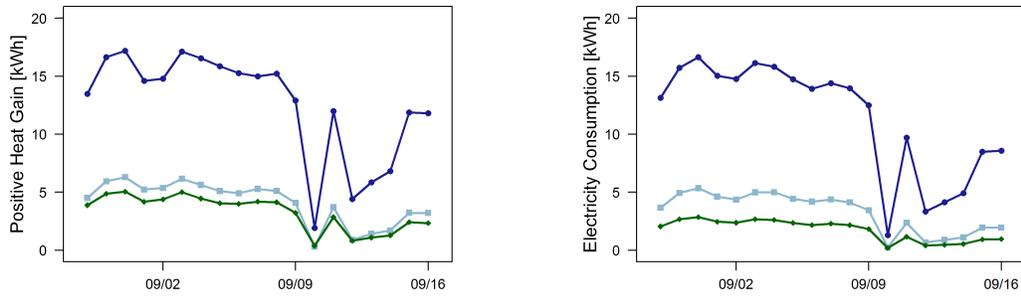
**FIGURE 8: Daily positive heat gain to conditioned zone and daily electricity consumption.**
