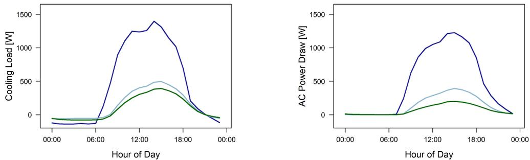
**FIGURE 9: Average cooling load and cooling energy consumption profile for 3 huts over 19 days.**
