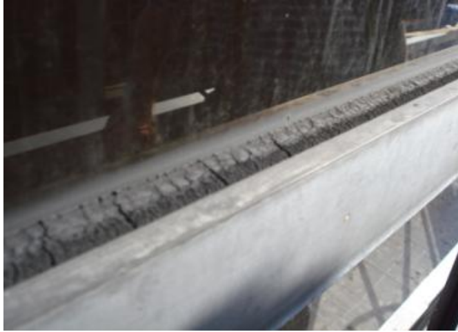
Photo 14 Example of aged gasket underperforming.
