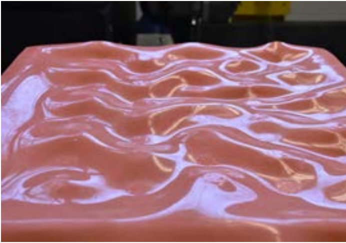
Figure 4. Flexible, reconfigurable deformable bed mold
