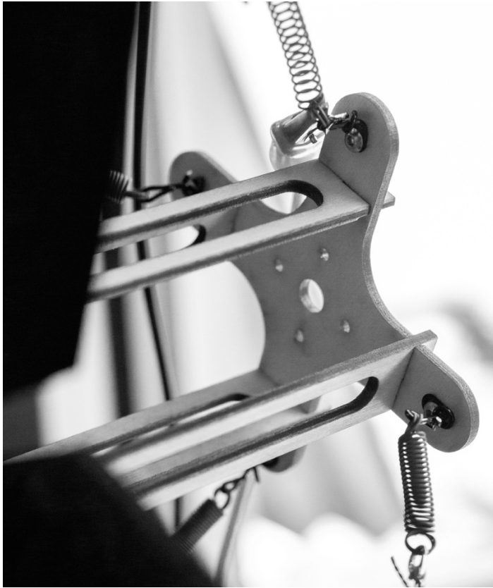
Figure 2: Actuation detail of kinetic system using Shape Memory Alloys.
