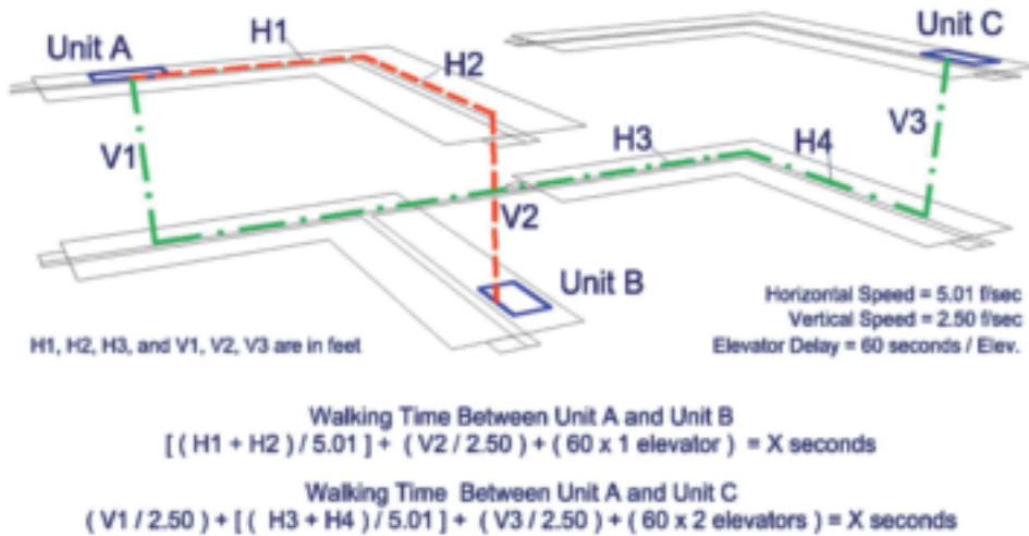
Figure 2 - Visual representation of the measurement method
