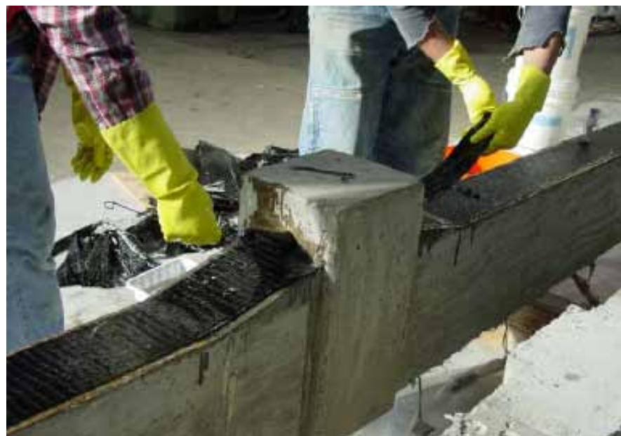
Figure 5. Carbon anchor through stub column. Image courtesy of Orton, S.L.
