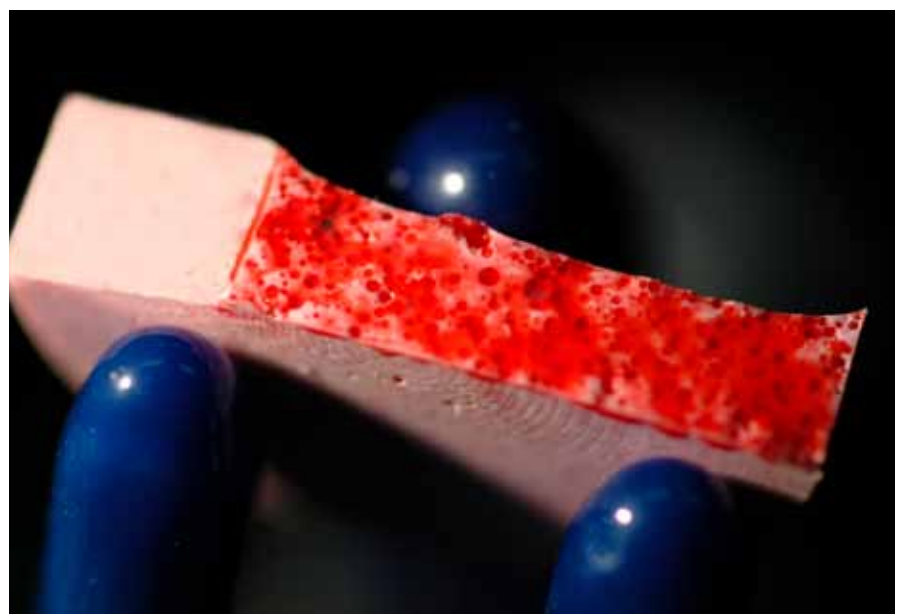
Figure 2. An example of a self-healing polymer, created at the Beckman Institute, University of Illinois.
