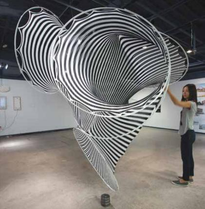
research builds upon the development of previous prototypes utilizing textiles manufactured on CNC knitting machines as the tensile surface in a textile hybrid system (figure 2).
