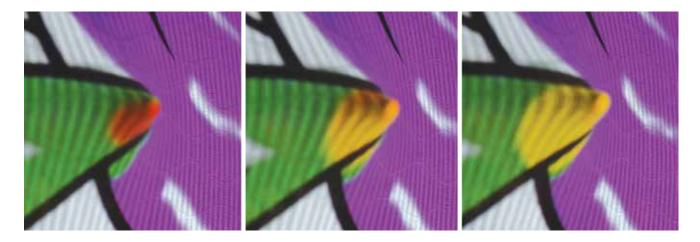
FIGURE 5. Size and color of the projection, at the point of interaction, changes from red to orange to yellow based upon the amount of pressure applied.
