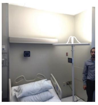
The experimental luminaire used to deliver the BWL (active) and DWL (inactive) interventions in participants' rooms.
