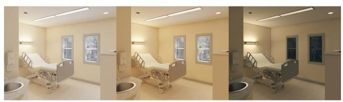
Figure 7: Simulations of hospital room lighting delivering high CS in the morning (left), medium CS in the afternoon (middle), and low CS in the evening (right).
