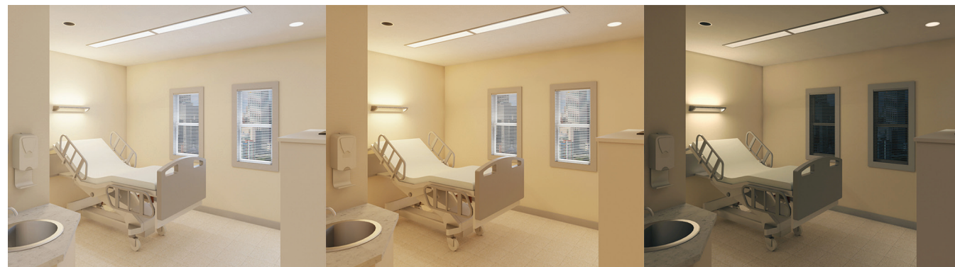
Figure 7: Simulations of hospital room lighting delivering high CS in the morning (left), medium CS in the afternoon (middle), and low CS in the evening (right).
