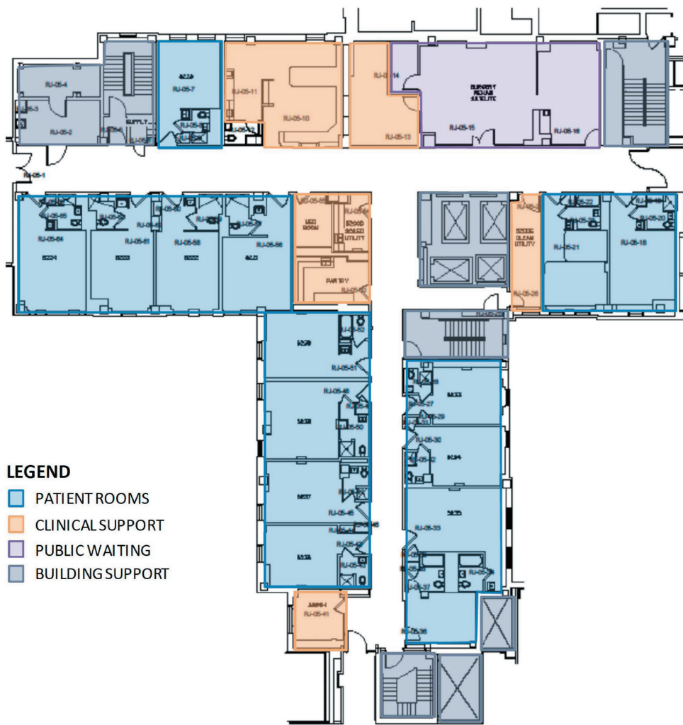
Figure 2. Existing floor plans of a 15-bed inpatient unit studied for conversion into a ‘safe unit.’
