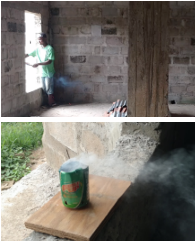
Figure 4. Soda Can Smoke Test. Photos by Author.
