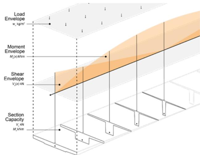
Figure 4. Structural analysis of a shaped slab.
