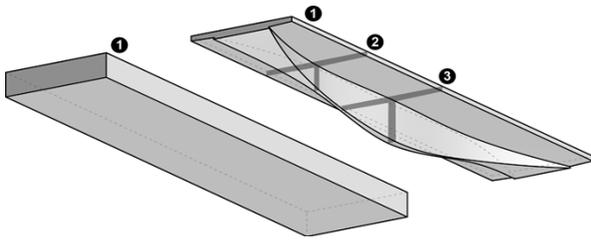
Figure 2. Overview of the design methodology: as opposed to the design of a prismatic slab where one section is designed for the maximum loading conditions, multiple sections are shaped according to the required capacity along the length of the slab.
