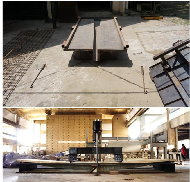
Figure 5. a) Disassembled curved sheet metal formwork for full-scale prototype with rebar shown to the right b) Load test configuration at NCCB in Faridabad, India, after the prototype was tested.
