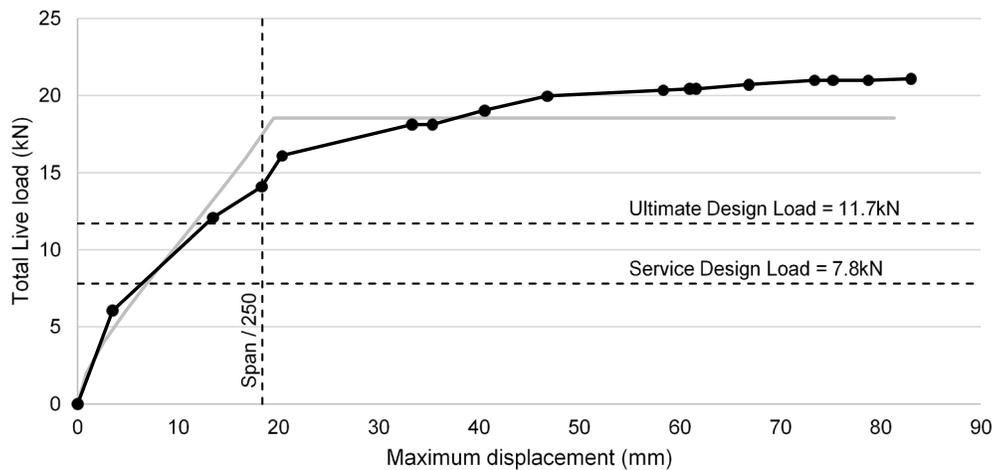
Figure 6. Load vs. displacement plot of prototype test, experimental results in black and predicted in grey.
