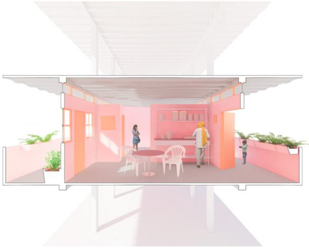
Figure 3. Rendering of multi-story construction built using shape-optimized concrete slabs.
