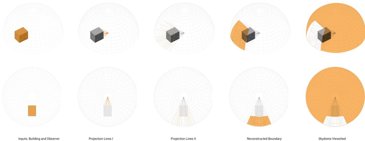
Figure 1. Spherical Projection Algorithm. Image Credit: POST-Project for Operative Spatial Technologies
