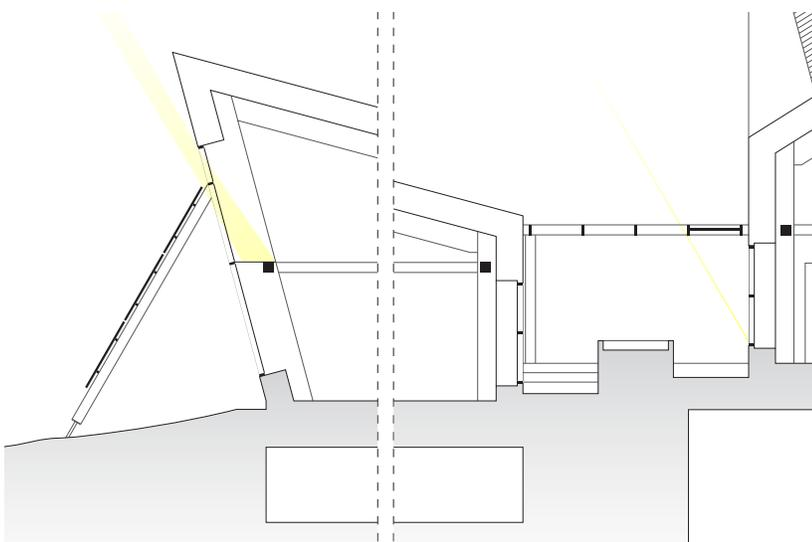
Figure 4c | Section Looking east with winter sun (60°) under Worst Case conditions
