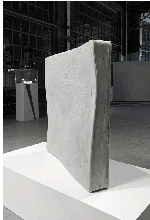
(left) Fig. 2 View of ribs behind panel, showing turning radius of the tool as well as geometries of the ribs, connecting at the turn. (right) Fig. 3 Panel that's printed face down, showing smoother surface from contact with mold. Note side edge has variable thickness where the back edge is flat to meet other building stock materials.
