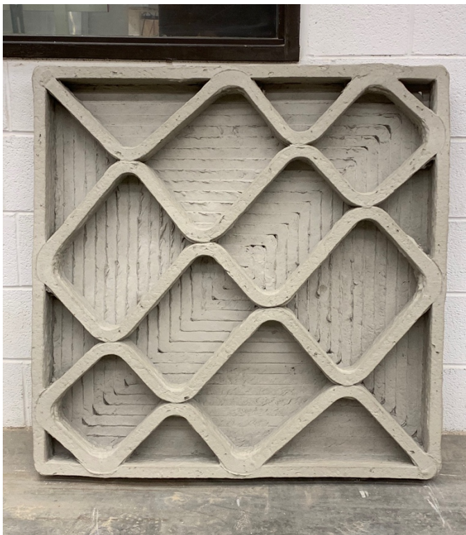
(left) Fig. 2 View of ribs behind panel, showing turning radius of the tool as well as geometries of the ribs, connecting at the turn. (right) Fig. 3 Panel that's printed face down, showing smoother surface from contact with mold. Note side edge has variable thickness where the back edge is flat to meet other building stock materials.
