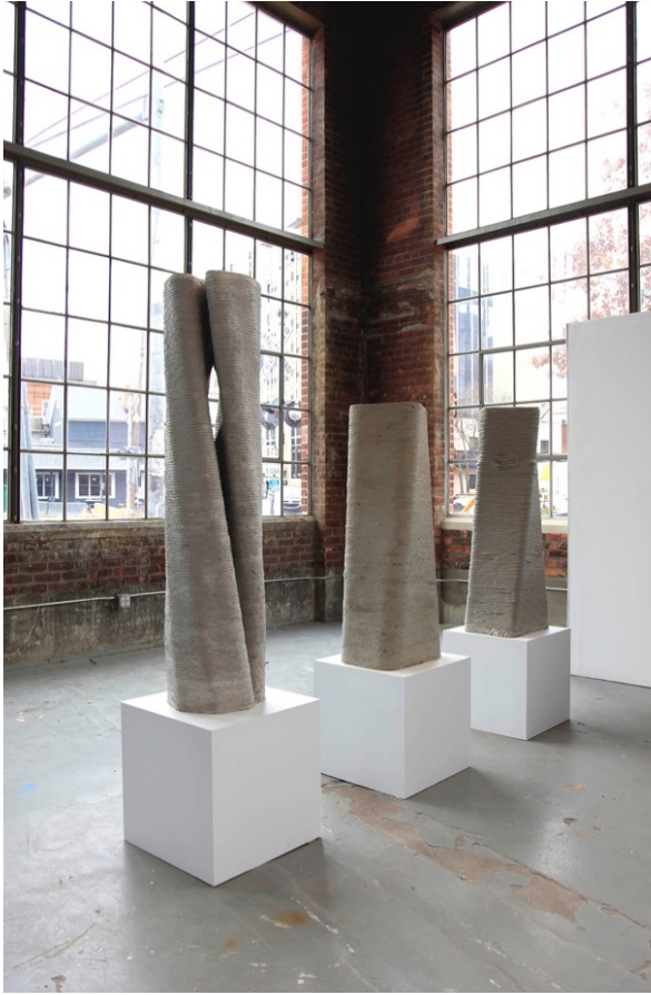
Fig. 4 Three columns showing progression of geometric complexity (from far right to left) and surface finish through bead shaping.
