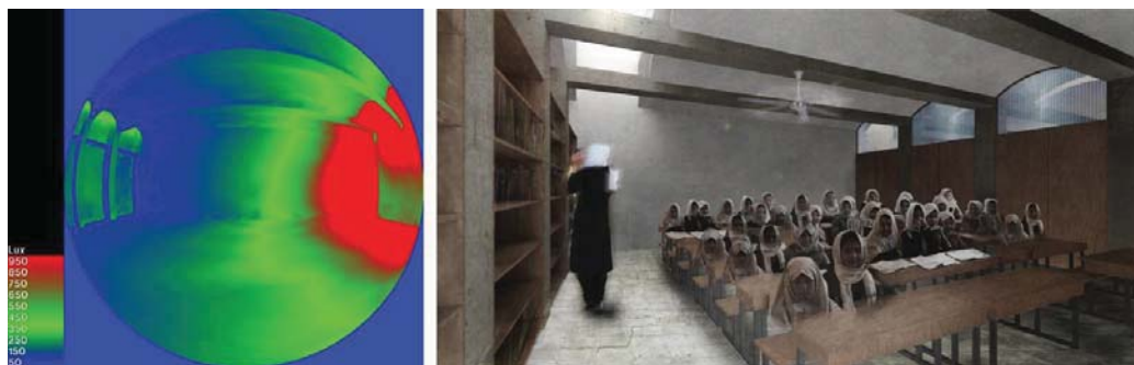
Figure 12: Optimized Afghan vaults create pleasant, daylit classrooms. Source: (Lang and Crofoot 2012)
