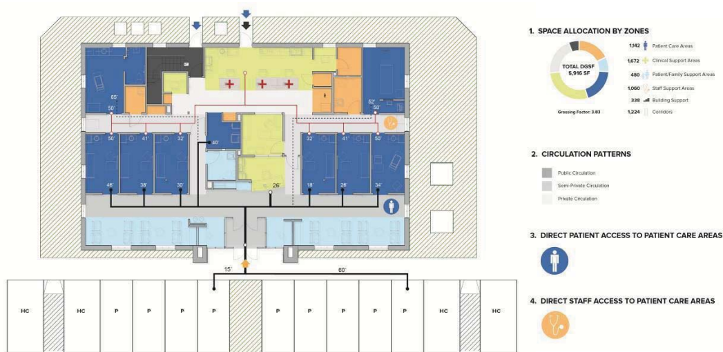
Figure 4: Post-occupancy evaluation analysis for workflow efficiency: clinical modules, circulation hierarchies and patient and staff travel distance
