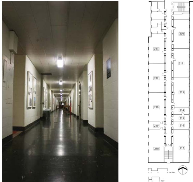
Figure 1: (a) Pacific Hall double-loaded corridor hallway; (b) Second floor plan of Pacific Hall with design studio classrooms and walls, called “breather corridor” containing the unused ventilation ducts.
