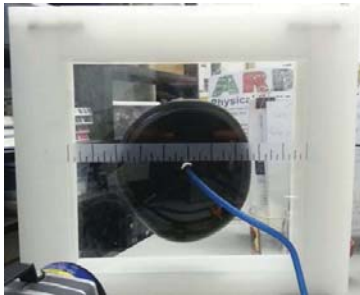
Figure 9: Latex balloon show inflated within the mock IGU
