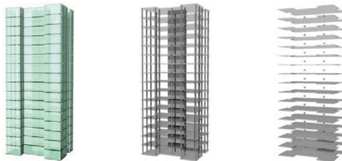
Figure 2: Example High Rise with glass curtain wall, concrete structure, and Agent Computing Mechanism (ACM) distribution
