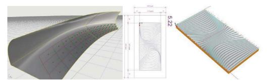
**Figure 12**: Left: Developable surface constrained by face normal angles, modeled in Rhinoceros; Middle: tool paths exported for use by RhinoCam; Right: Simulation of panel surface stock for CNC routing. Source: (Author 2013)
