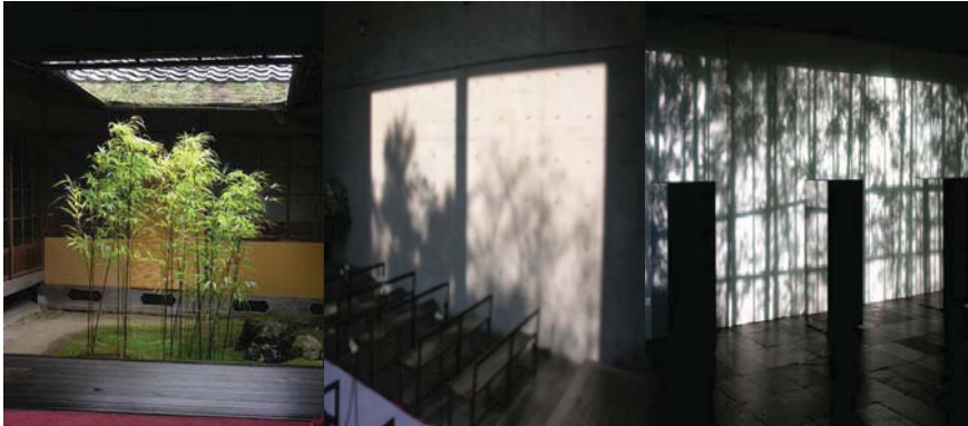
Figure 1: Three methods of effectively bringing weather-generated outdoor movement indoors without compromising the weather-roof envelope of a building. From the left: enclosure in an internal court; sunlight projection onto an interior surface; and back projection onto a translucent external cladding material.
