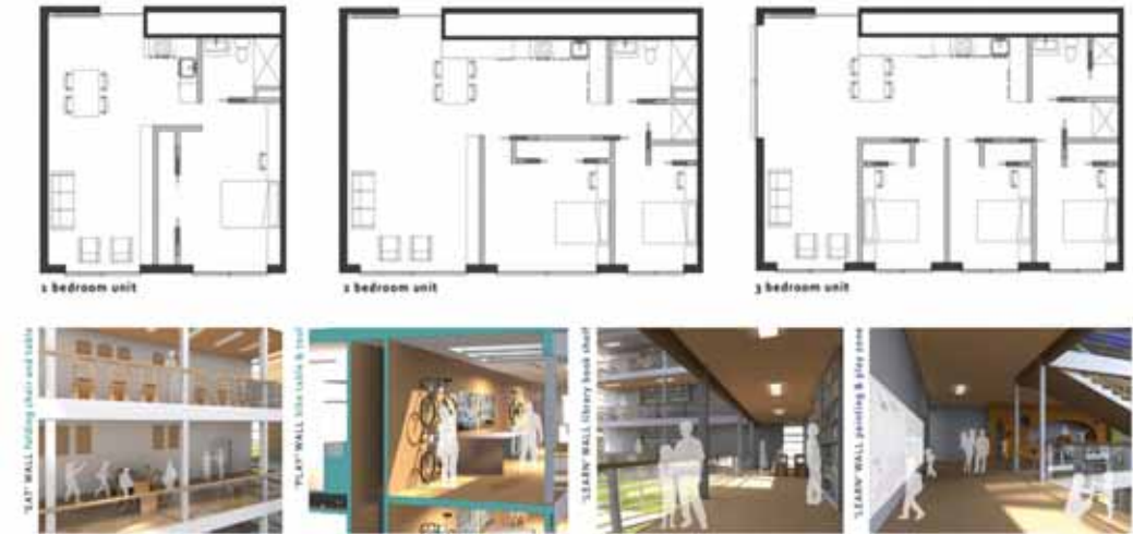
Figure 5: Floor plans and smart-wall concept from “knot” project. Source: (Atria and Kim 2013)
