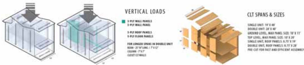
Figure 7: Load Paths and panel sizing from “seed” project. Source: (Boulier and Boykin 2013)
