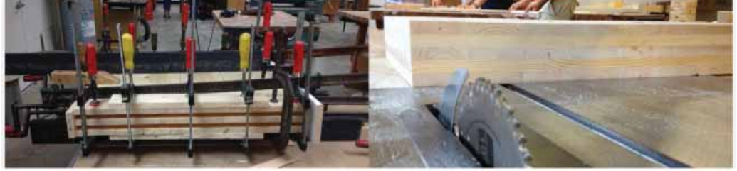
Figure 2: CLT material study from “treaty oak” project. Source: (Barrett and Martin 2013)
