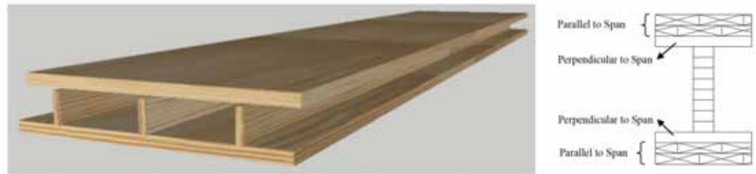
Figure 9: Long-span hmt panel. source: (montgomery, et al. 2014)
