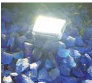
Figure 7: The sensor placed on the glass material wrapped in aluminum paper.
