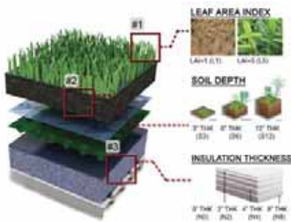
Figure 12: Various parameters that would be used in this research are shown in the section of green roof
