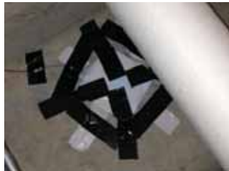
Figure 9: Thermocouples affixed to the concrete sub-slab beneath each roof section.
