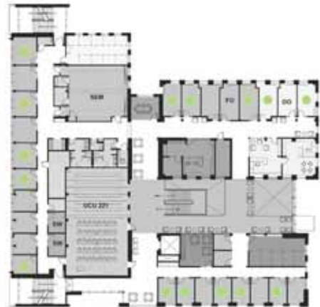
Figure 5: Datalogger locations on the second floor
