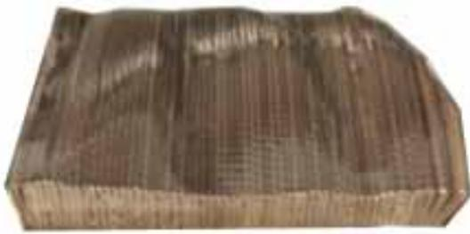
Figure 2: Plexi Vacuum formed on cardboard (Smith 2014)
