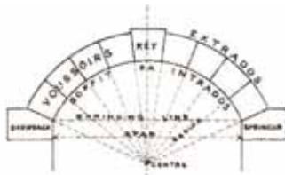
Figure 2: Segmented arch with defined terms: (Purchase 1904)
