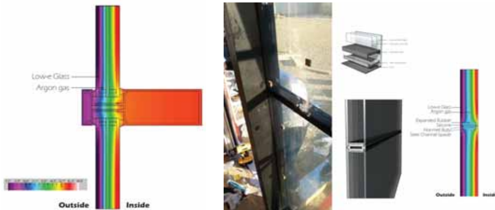
Figure 2: Manko's 250i system with triple glazing and thermal break (left) and System A prototypes and thermal simulation. Source: (Author 2014)
