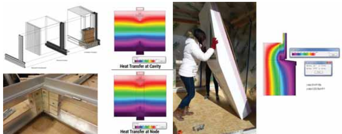
Figure 3: System B diagrams and thermal simulation (left) and System C prototype and thermal simulation (right). Source: (Author 2014)
