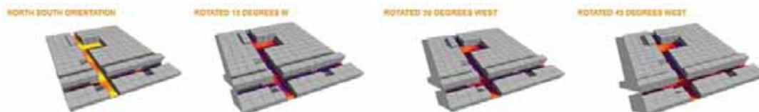
Figure 8: Outdoor solar analysis: four orientations in Eden City Mall
