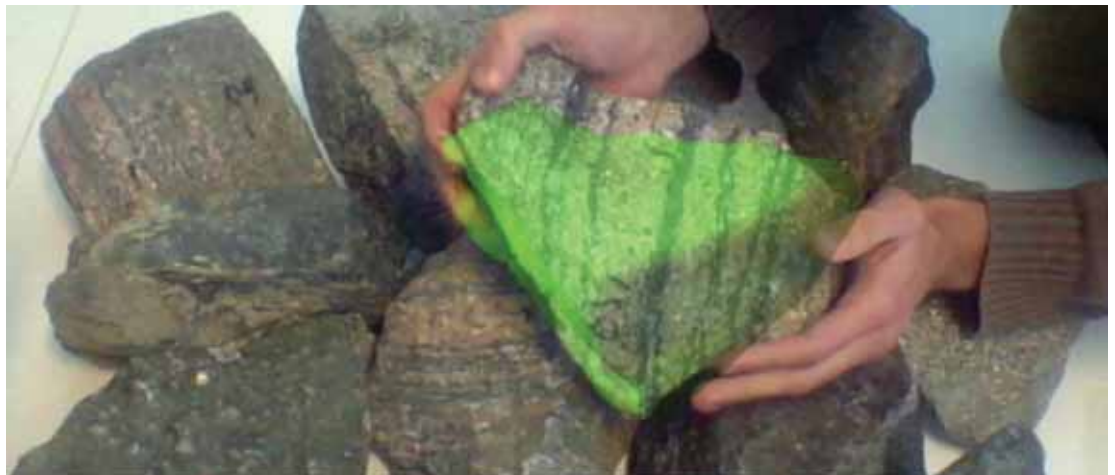
Figure 14: Augmented mesh model of stone shown on top of existing conglomerate of stones.
