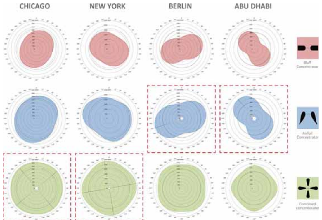
Figure 10: Energy production profile as functions BIWT alignment, the most efficient BIWT in each city is shown in a dash line rectangles. Also the best orientation of BIWT is shown with white arrows.
