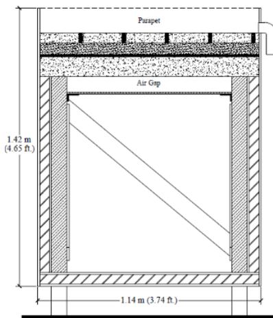
**Figure 2:** Test cell structure section
