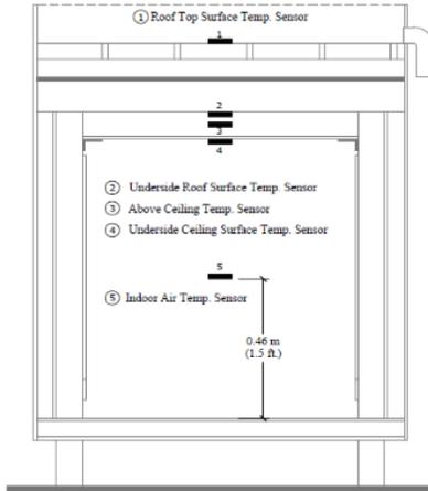
Figure 3: Sensor placement
