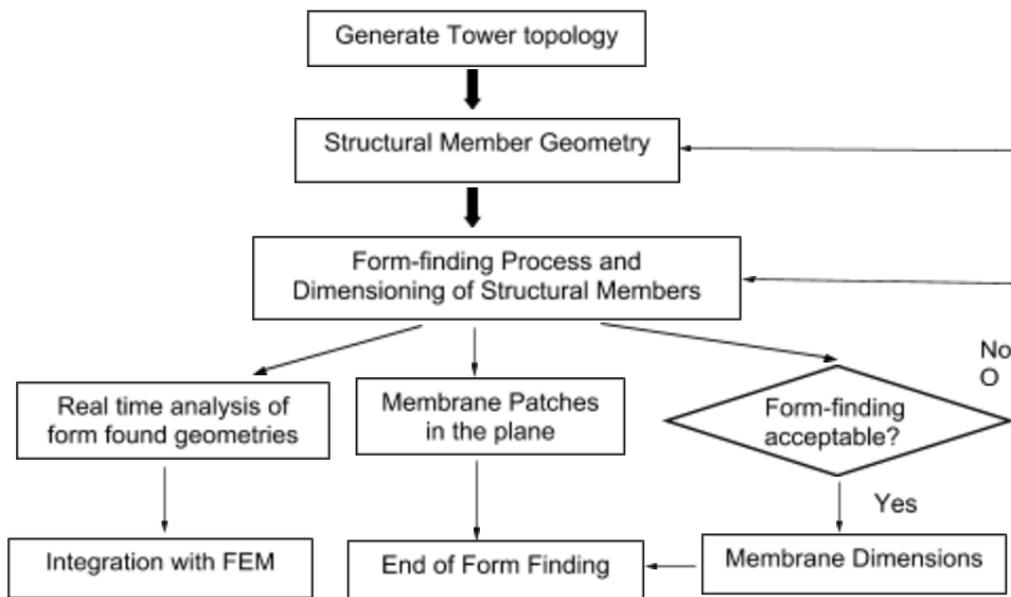
**Figure 5:** Form-finding process (adapted from Holden Deleuran et al, 2015)
