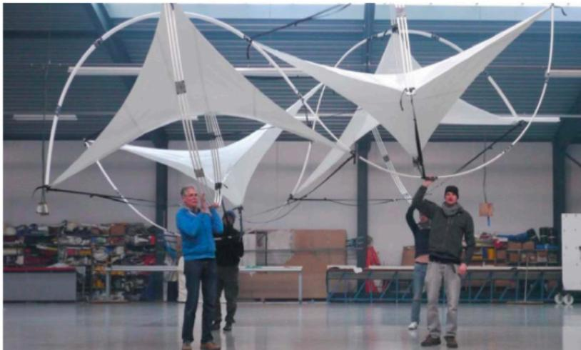
**Figure 3:** Bending-activated tensegrity structure (Schling et al 2015, reprint with permission)
