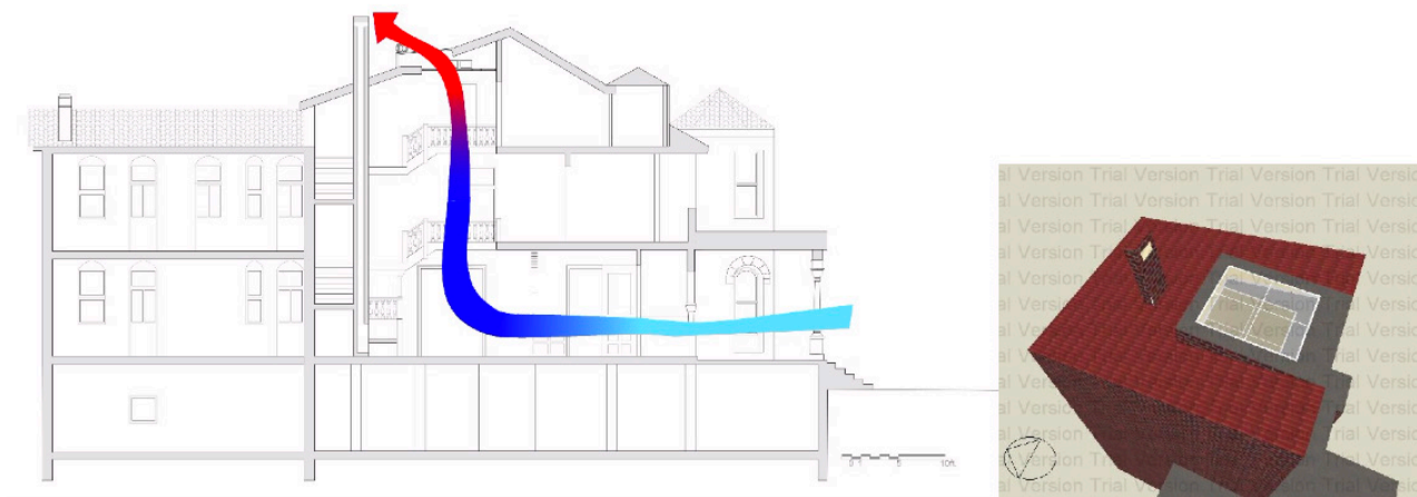
Figure 6 and 7: Diagrammatic section through the Kalteyer house (Author, 2016) and the Design Builder whole building performance model.
