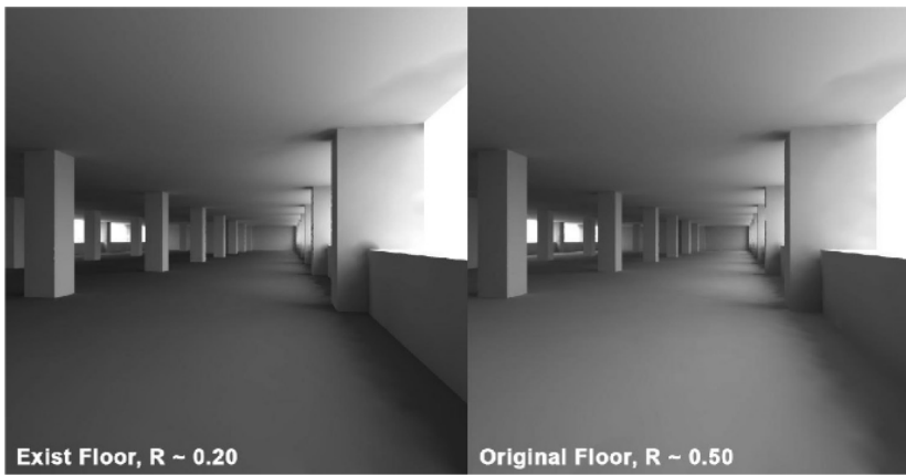
Figure 6: RADIANCE visualizations in a typical floor, without blinds. The image at left shows the existing floor, a dark carpet; the image at right shows a more reflective floor like that originally used in the building. The sky condition for the simulation was overcast. (Source: Author)
