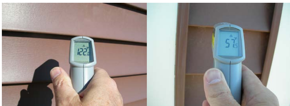
Figure 3 65F Delta T, Vinyl Siding in Full Sun and Shade on a 57F Day
