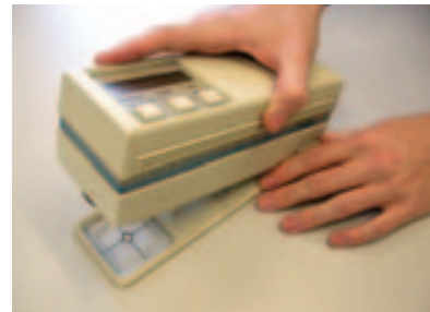
Figure 2.23 An example of a commercial portable spectrophotometer for measuring colour
