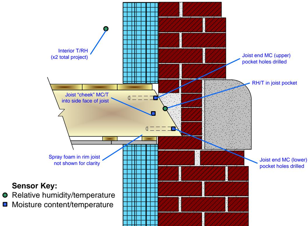
**Figure 6: Schematic of typical joist end sensor monitoring package**
