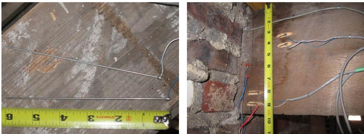
**Figure 7: 6” extended moisture content pins (left) and installed moisture content pins (right)**
