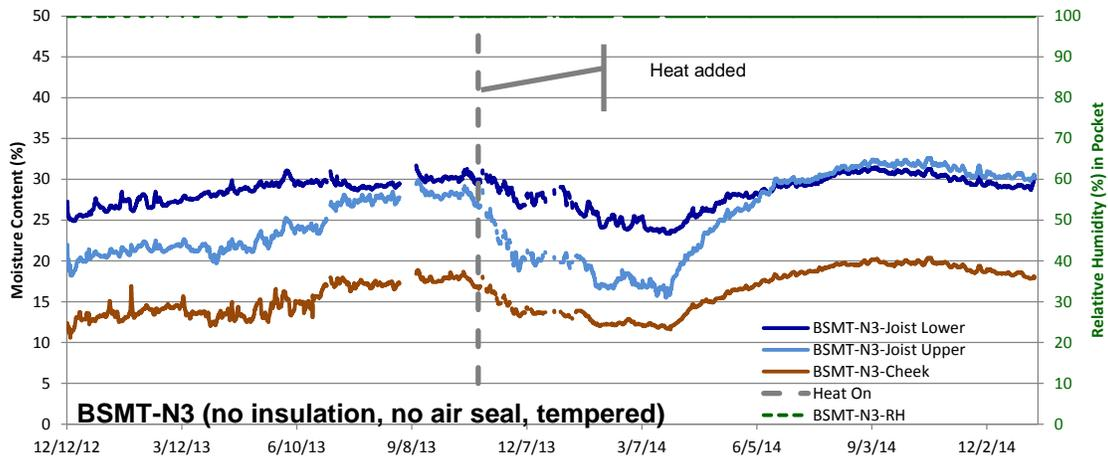
**Figure 11: Basement North 3 (uninsulated) joist end moisture contents and relative humidity**
