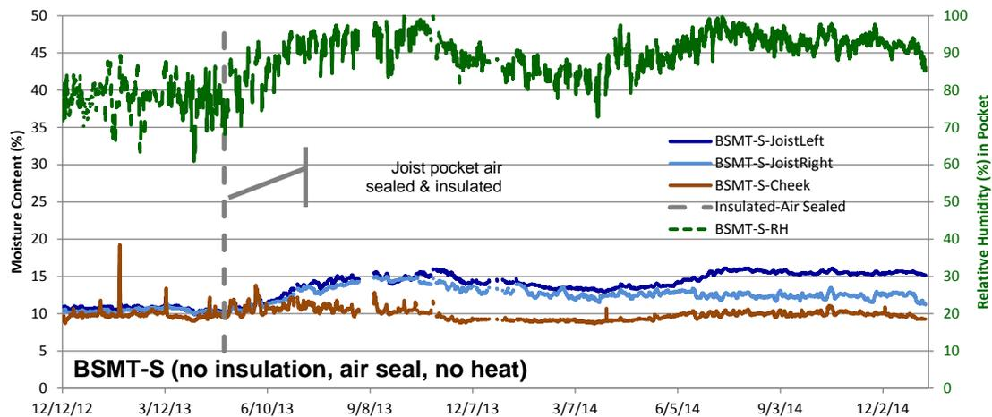
Figure 12: Basement South joist end moisture contents and relative humidity
