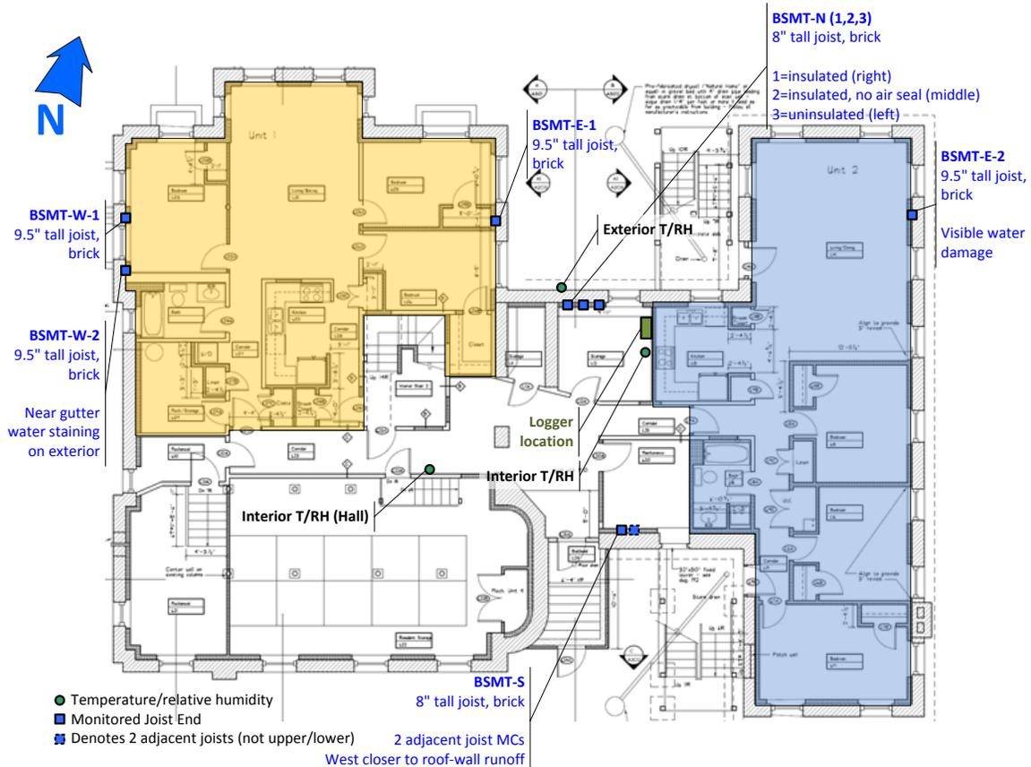
**Figure 4: Location of monitored joist ends at basement level (basement ceiling)**
