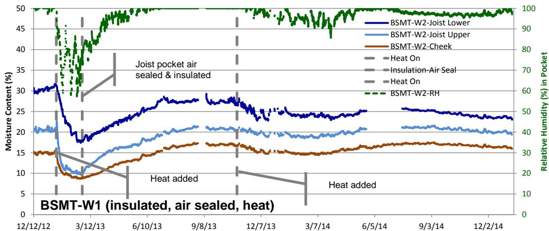
**Figure 14: Basement West-2 joist end moisture contents and relative humidity**
