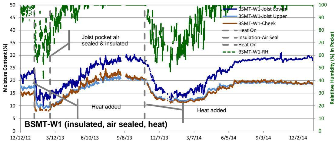
**Figure 13: Basement West-1 joist end moisture contents and relative humidity**
