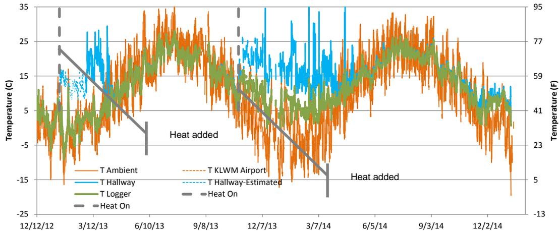
**Figure 8: Exterior and interior temperatures; with airport (KLWM) temperature data**
