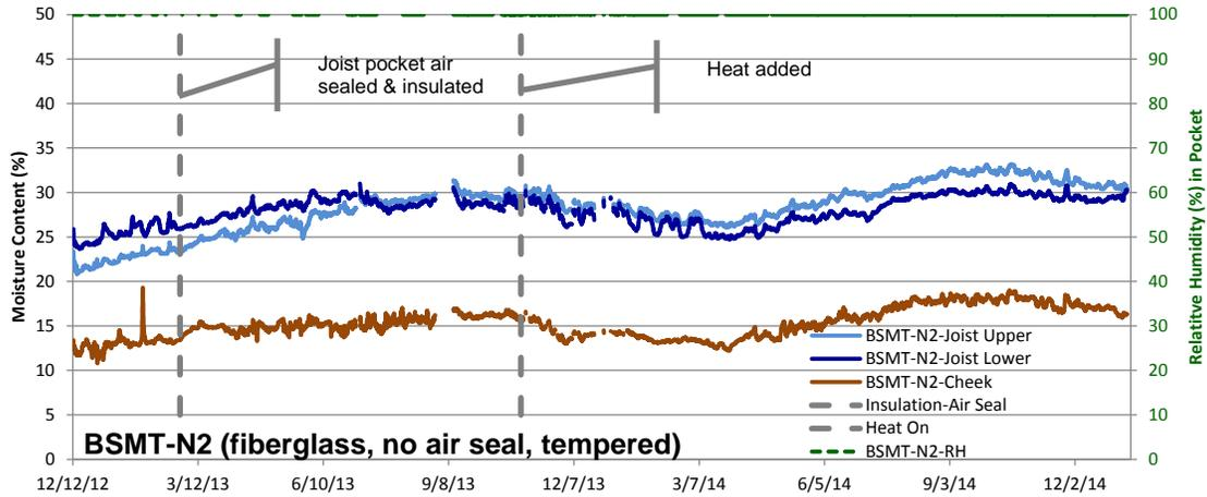
**Figure 10: Basement North 2 (fiberglass) joist end moisture contents and relative humidity**
