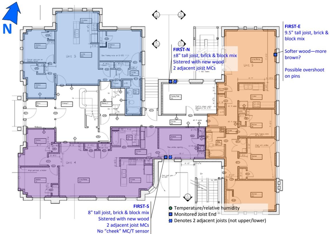
**Figure 5: Location of monitored joist ends at first floor (first floor ceiling)**
