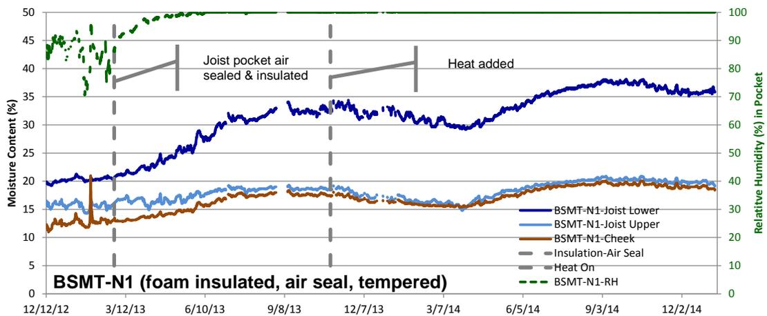
**Figure 9: Basement North 1 (insulated) joist end moisture contents and relative humidity**
