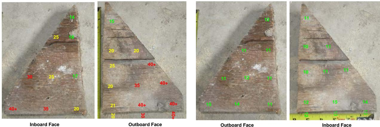
**Figure 15: Joist end moisture contents for southeast (left) and southwest (right) corners**
