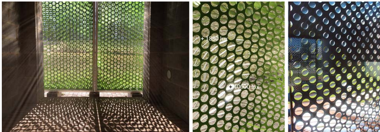
FIGURE 7. Full-scale component prototype of Eclipsis ™ system: a) left image shows component prototype being field measured in a test cell, b) center image shows reflected glare on stainless steel disks and c) right image shows view of Eclipsis ™ from LumenHAUS interior
