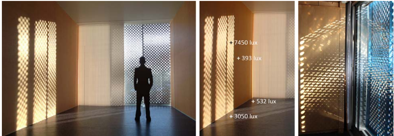
FIGURE 6. Test cell observations of Eclipsis ™ system: a) left image shows photographic survey of scaled physical model, b) center image shows photometric readings in scaled physical model and c) right image shows reflected and direct solar gain observed in LumenHAUS
