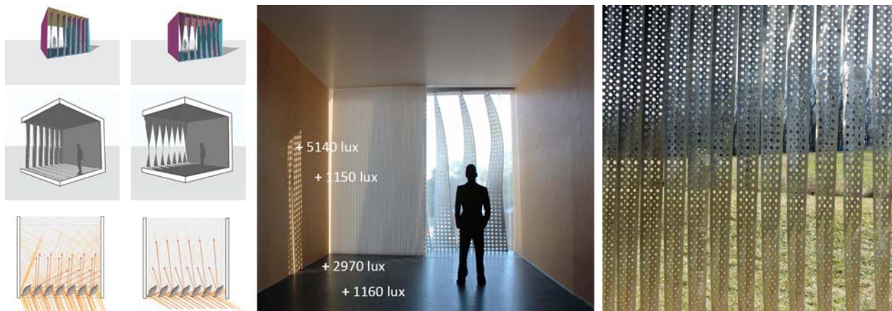
FIGURE 9. HDLR development of metal ribbon prototype: a) left images show multi-state simulation, b) center image shows photometric measurements of the scaled physical model and c) right image shows testing of the component prototype
