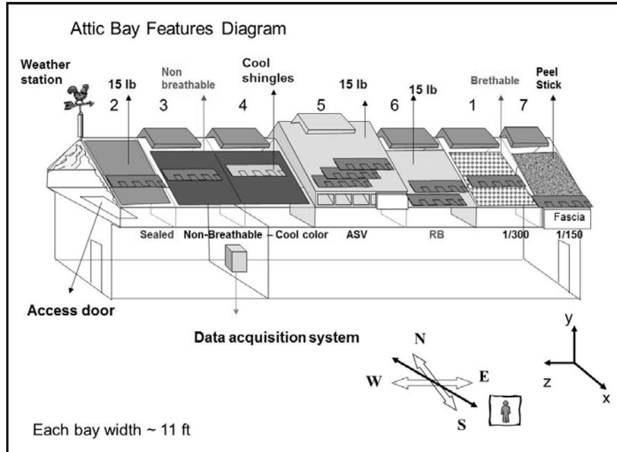
Figure 2: Test attic assembly layout on NET Facility in Charleston SC.
