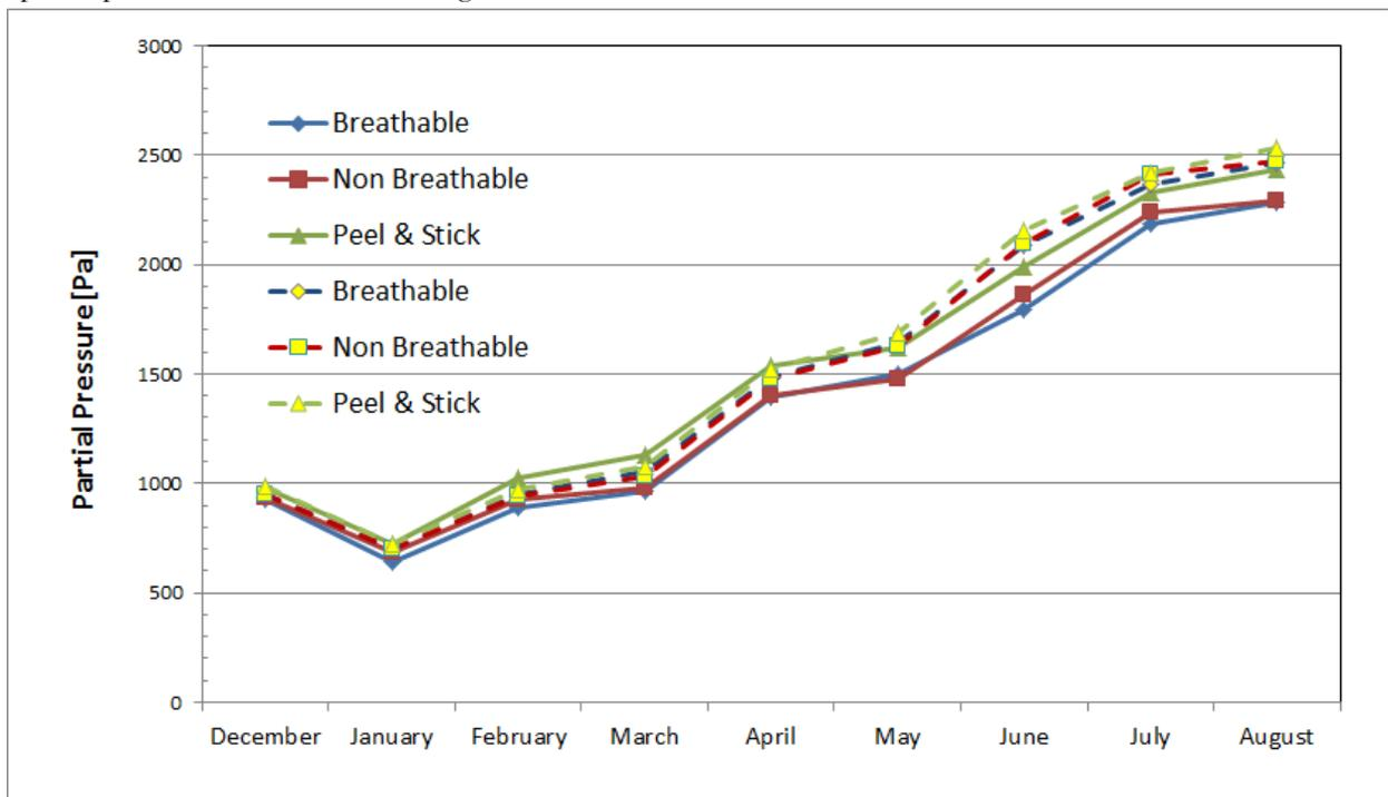
Figure 5: Roof-deck and underlayment moisture represented by the partial pressure of the water vapor computed from temperature and relative humidity measures made at the top-side and underside of the sheathing.
