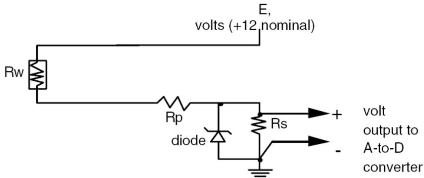
Figure 4. Circuit to measure resistance of wood with DAS.
