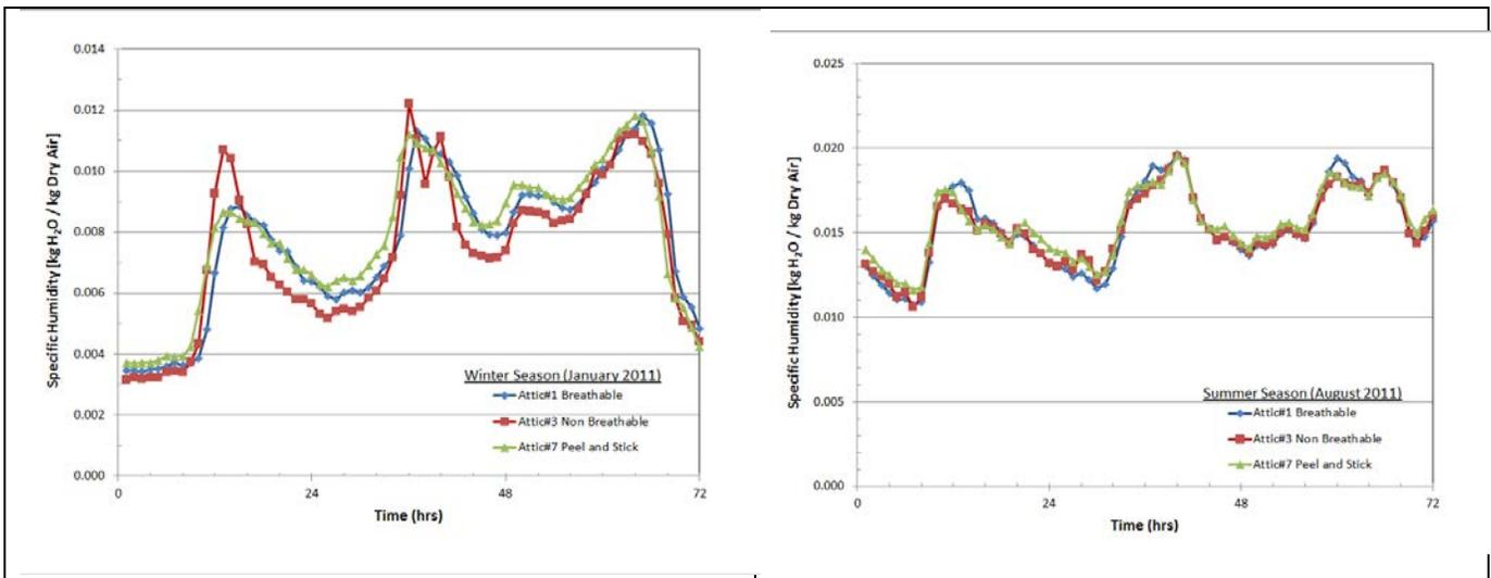
Figure 6. Moisture in attic air for a typical week in winter and summer under study at NET facility.
