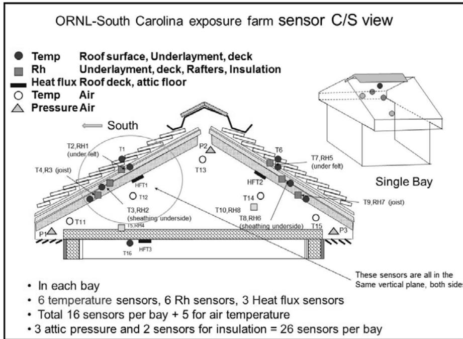
Figure 3: Instrumentation layout for each attic assembly
