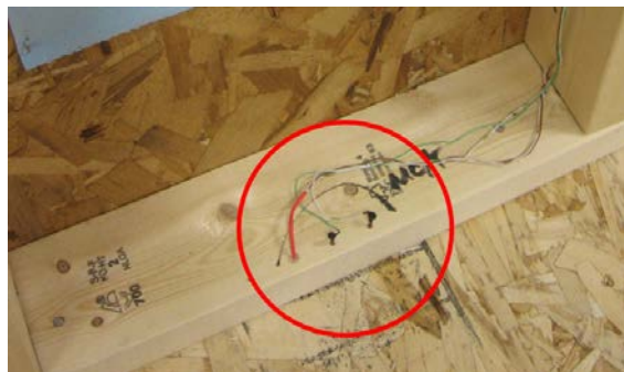
FIGURE 6: Moisture Content Sensor at Interior Edge of Bottom Plate
