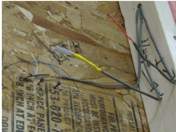
FIGURE 1: Sheathing MC/T and Cavity Space RH at Mid-Depth and Interior Temperature-Only Sensor for Walls 3a and 3b
