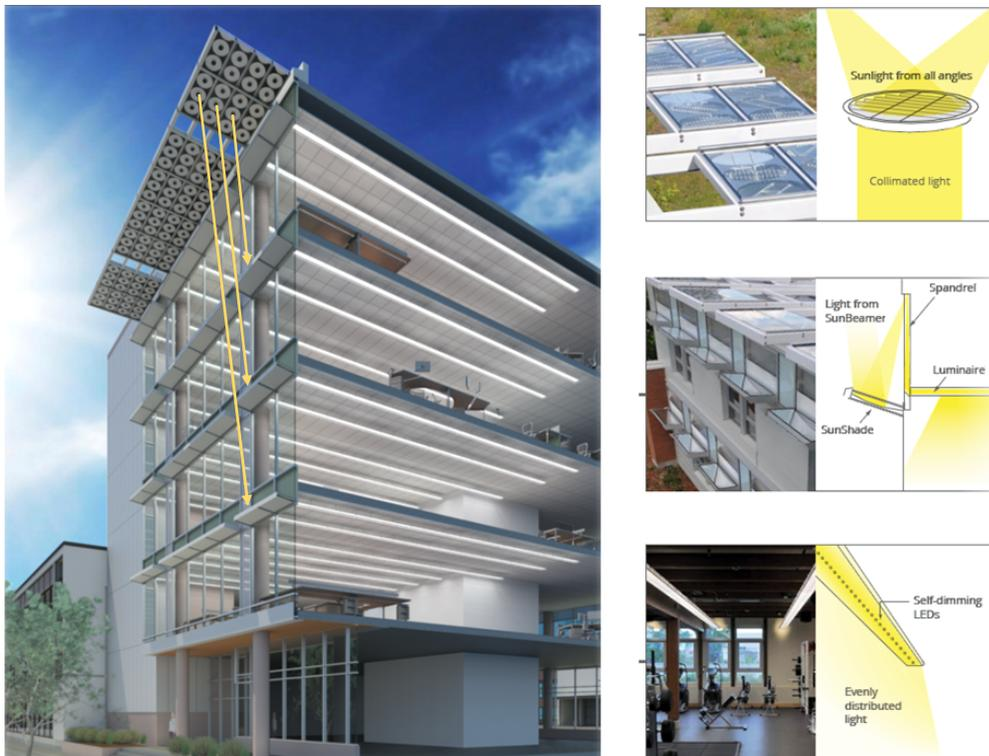
FIGURE 1: Active daylighting system showing the integrated components that collect and distribute sunlight deep into multi-story buildings. Image courtesy: SunCentral Inc.
