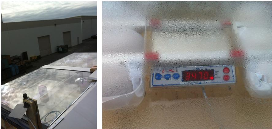
FIGURE 15: Prototype photos E1 at bottom left, E2 at top left and the desiccant and scale in E2 (right image). Condensation visible on the enclosure was on the outside of the glass.
