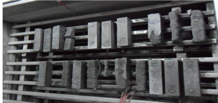
*The samples of series F-01,F-02,F-05 and F-06 after 100 freeze-thawing cycles*
