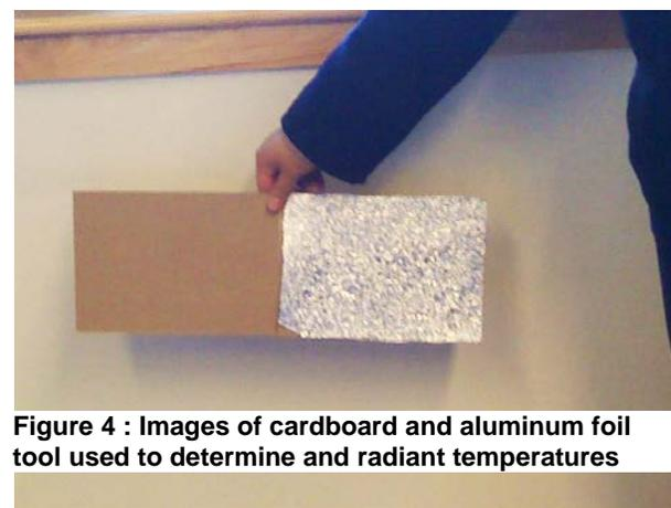
Figure 4 : Images of cardboard and aluminum foil tool used to determine and radiant temperatures
