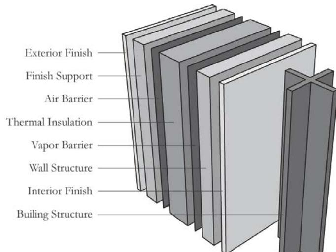
Figure 1: Diagram of Current Layered Facade Construction
