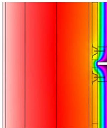
The joints were revealed to be the key difference between metal panels that perform poorly and those that performed well. In the poor performing options, the metal front of the panel wraps through the joint, providing a thermal bridge that greatly undermines performance. The façade that performed well, in both the infrared image and the simulation, was backstopped at the gap between connecting panels. The backstop was made of insulation which was
