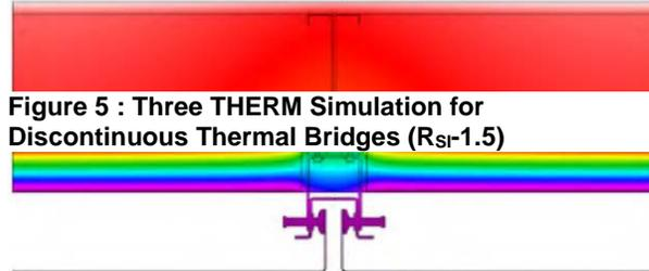
Figure 5 : Three THERM Simulation for Discontinuous Thermal Bridges ( $R_{SI}=1.5$ )
