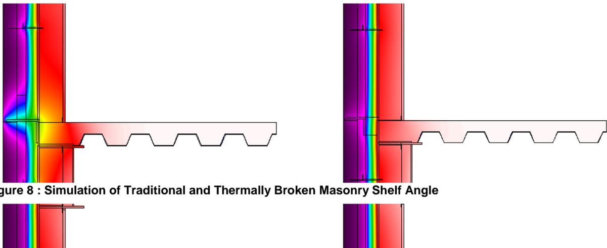
Figure 8 : Simulation of Traditional and Thermally Broken Masonry Shelf Angle
