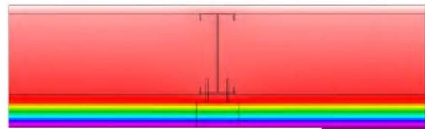
Parallel Path Simulation with Thermal Bridge ( $R_{SI}=0.6$ )
