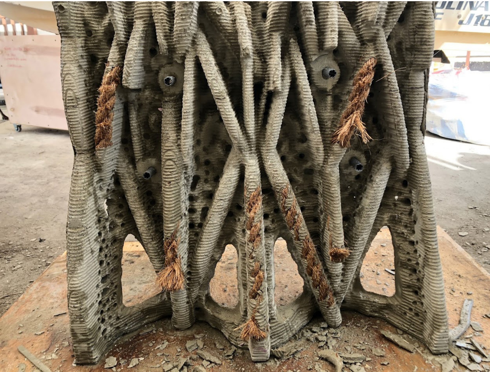
Figure 31. Half-scale prototype panel testing a double-sided mold and embedded ropes.
