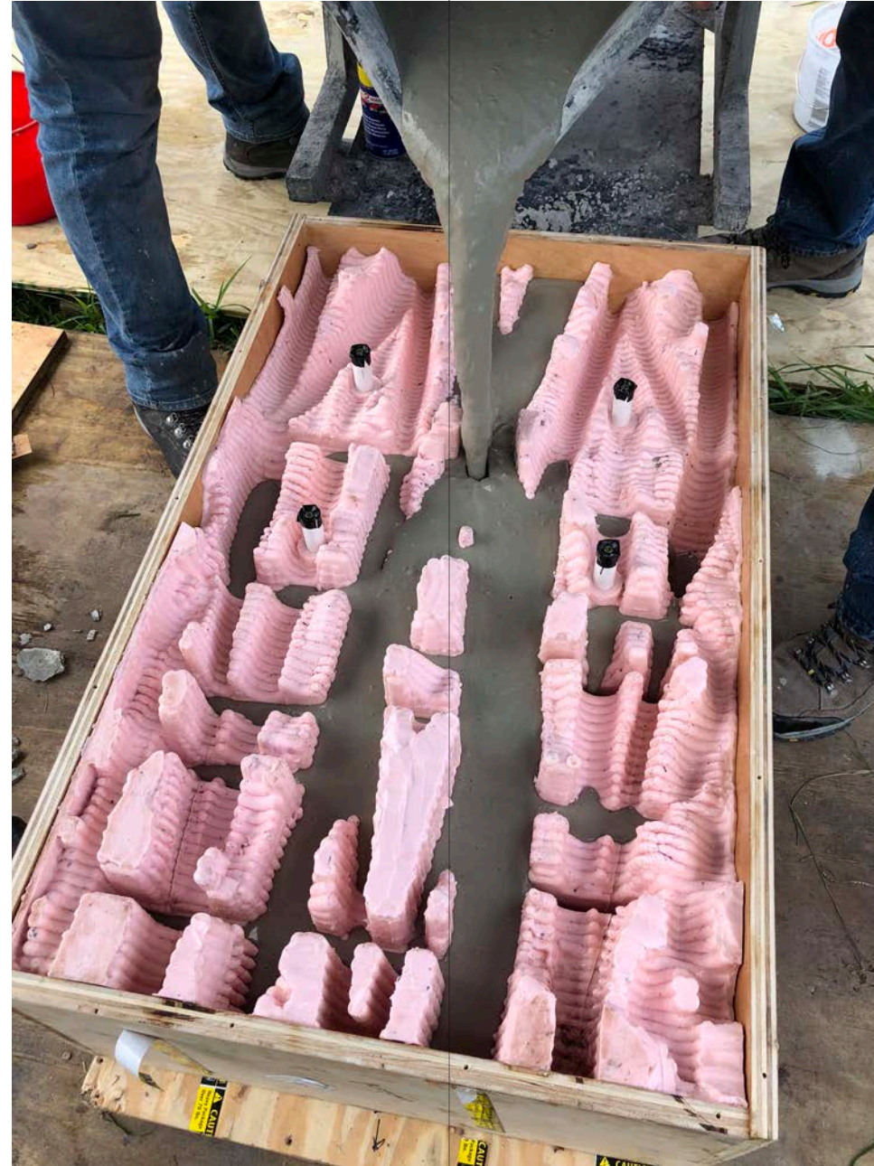
Figure 23. Panels for the Fort Pierce installation were 24"x36" and cast with a silicone rubber mold. Roots extended approximately 12" outward from the seawall face. Oyster flour (above left) was added to the concrete mix to be marine-friendly.
