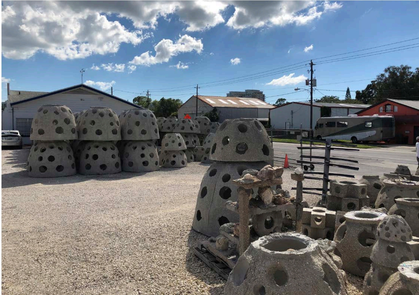
Figure 14. Reef Ball Foundation operates a facility in Sarasota, FL that produces a variety of shapes and sizes of artificial reefs.
