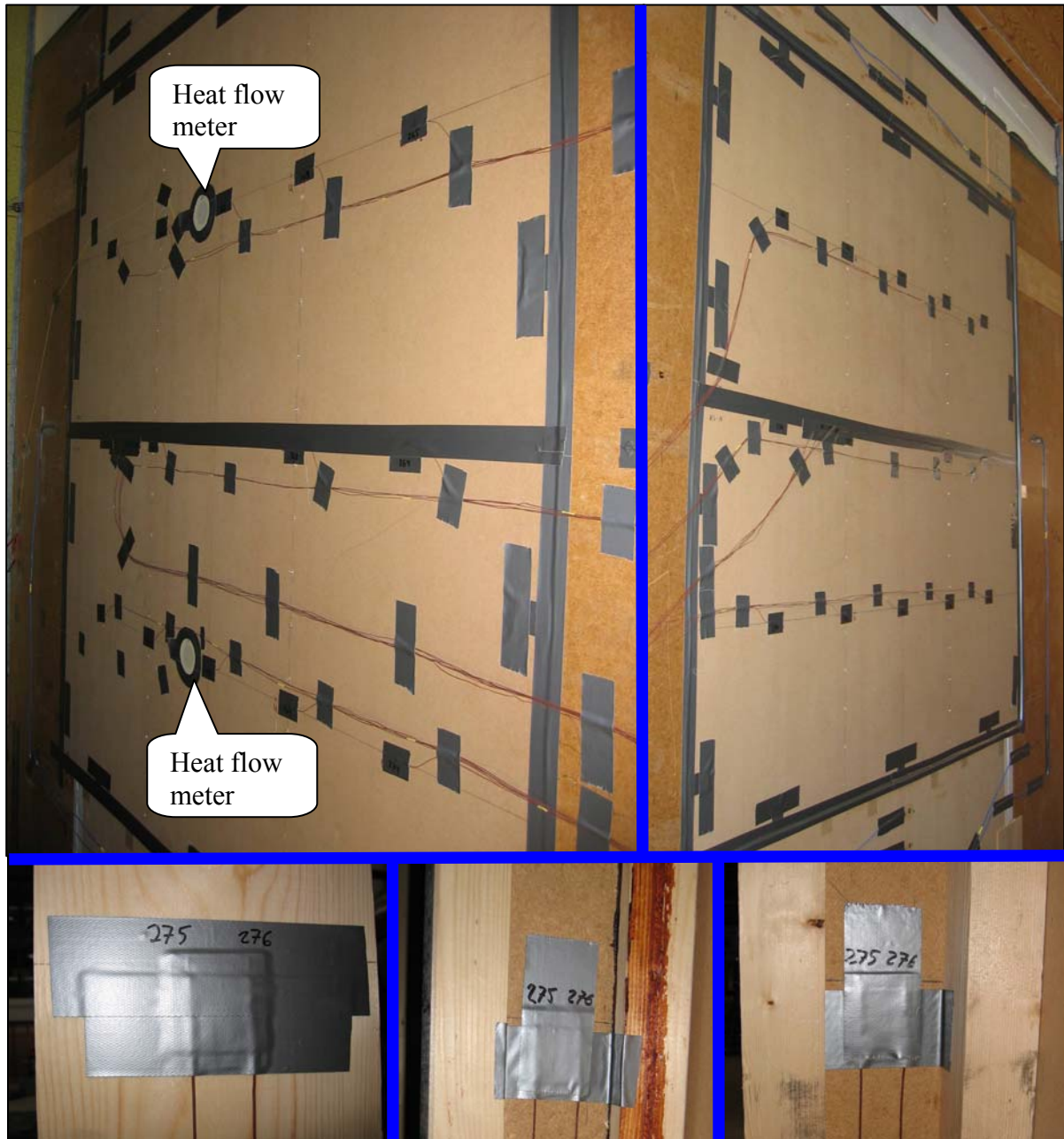
Figure 2-5 Placement of thermocouples and heat flow meters on wall and studs. Upper left: Hot side, Upper right: Cold side. Lower left: 36 mm stud, Lower middle: I-stud, Lower right: U-stud.
