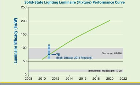
continue to improve. By 2015, LED luminaires (fixtures) will be capable of luminaire efficacies exceeding 150 lm/W, more than twice that of a typical fluorescent fixture. Lowering the drive current applied to the LEDs can increase efficacy. The high-efficacy 2011 products shown on the graph achieve 75 lm/W using a standard drive current, but there are other high-efficacy products on the market that range from 60 lm/W to 110 lm/W, depending on the drive current.
