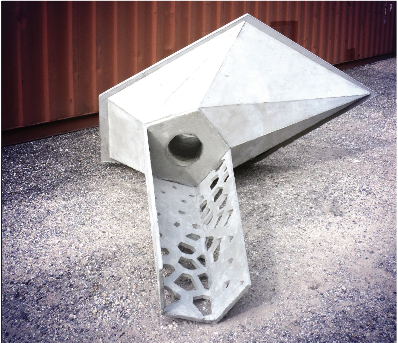
Figure 4: Single Rhizolith Island element, 10-20 of these elements make up one island (Source: Author).
