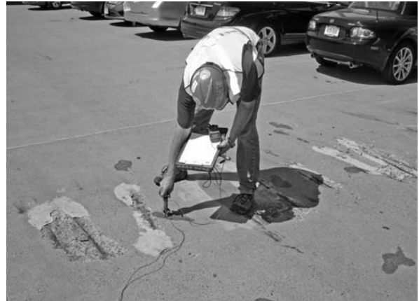
▲ Half-cell potential readings can be used to identify areas of reinforcing steel that are at greatest risk of corrosion.
