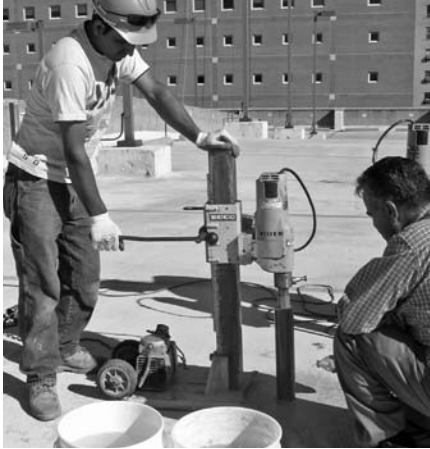
▲ Core samples of concrete may be tested for chloride content, strength, and composition to guide the design professional in evaluating the structure's resistance to corrosion.
